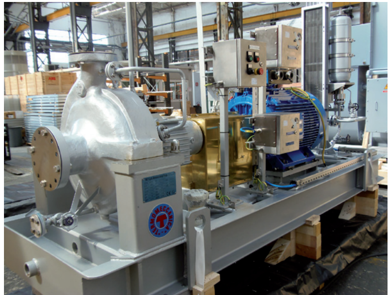
Fig. 2 - Export pipeline booster pump (OH2)
