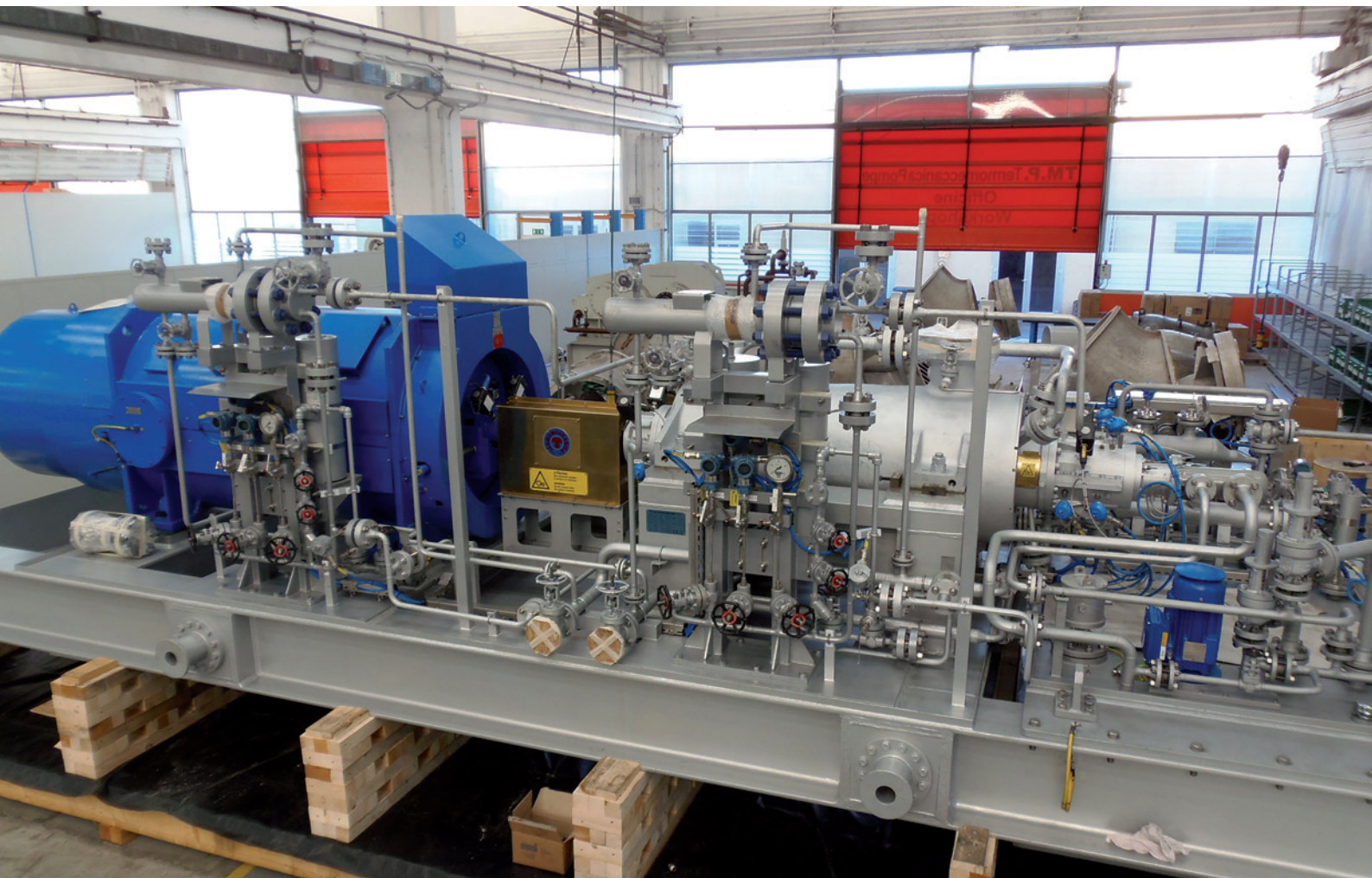
Fig. 1 – Export oil pipeline pump (BB5)
